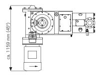
Weight according to equipment (without motor) approx. 515 - 680 kg (1135-1500 lbs.)
